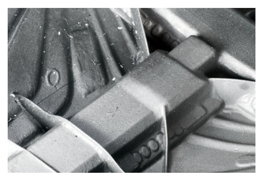
**Face Welds** - many of you are aware, like the crown, a driver's face is a separate piece that must be welded, brazed, or otherwise attached to the body. Some manufacturers and models, as you'll see, have cleaner welds than others.
