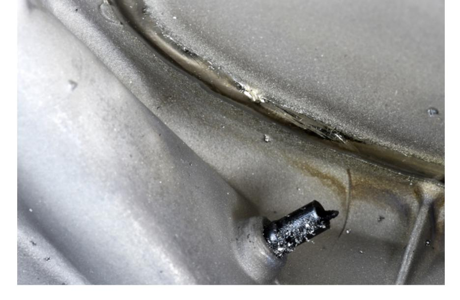
**Hot Melt** (the blob of goo you see in some of the heads) - Holt melt was fairly common in the days of bonded hosels where it was used to catch any bits of epoxy or other debris that might come loose and would otherwise have rattled around in the head. Hot melt is still used for that purpose, but it's also used to help heads make weight if they come up a little light. Finally hot melt is used to tune the acoustics in otherwise unpleasant sounding heads.
